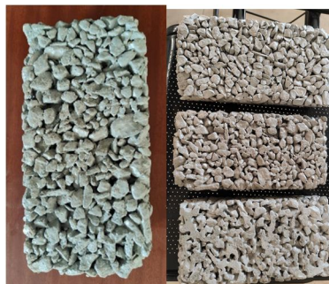
Figure 3 Permeable Concrete pavement block after curing.
