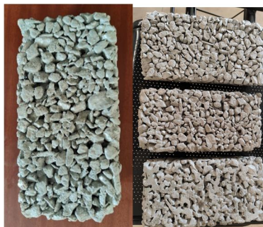
Figure 3 Permeable Concrete pavement block after curing.
