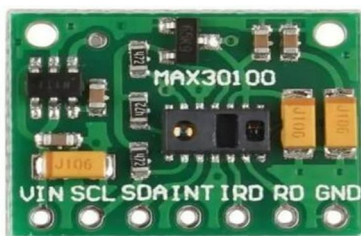
Fig 3.3 MAX30100 integrated pulse oximetry and a heart-rate sensor.
