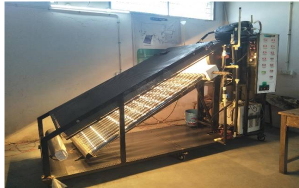
Fig. 1. Evacuated Tube Collector Characterization System
