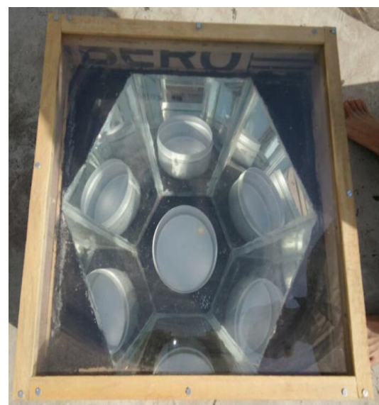
Fig. 4: Hexagonal Solar Cooker
