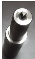
Fig. 2 Triangular tool pin profile
