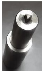
Fig. 2 Triangular tool pin profile
