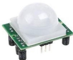
Fig. 3 PIR Motion sensor
