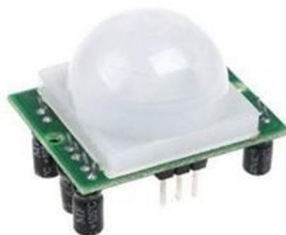
Fig. 3 PIR Motion sensor
