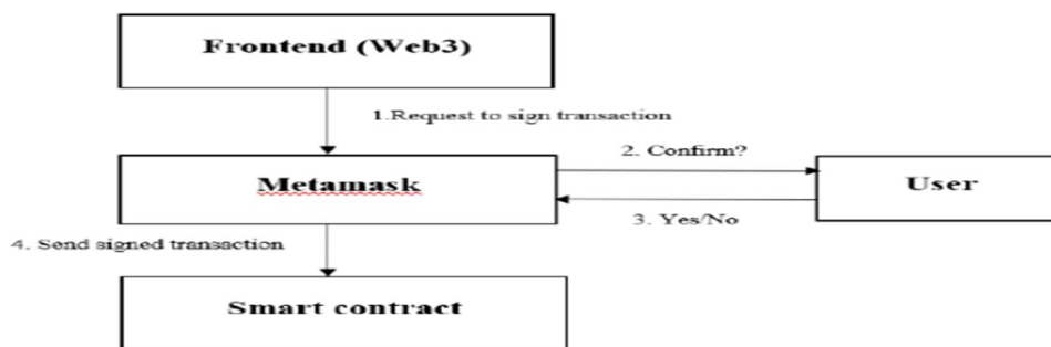
Fig. 3. Working of Smart contract
