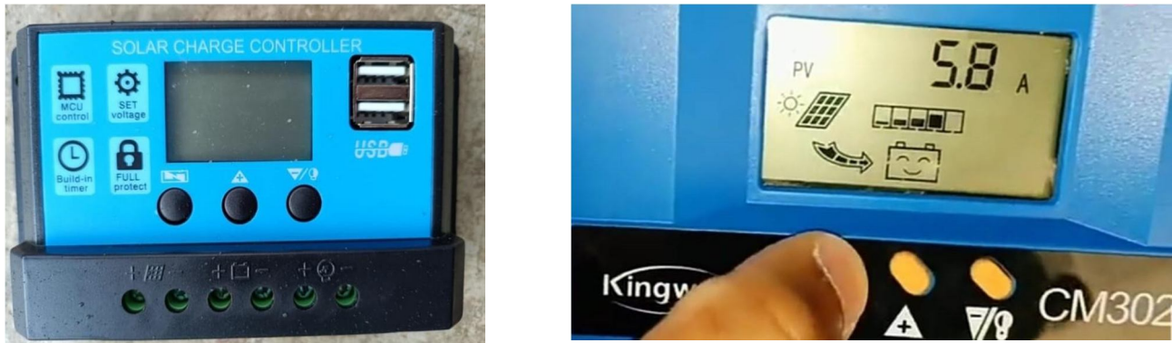
6. Solar charge controller
