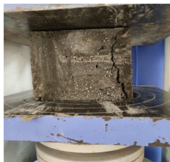
Fig 1.6 Performing Compression Testing
