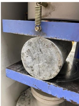
Fig 1.6 Performing Split Tensile Testing
