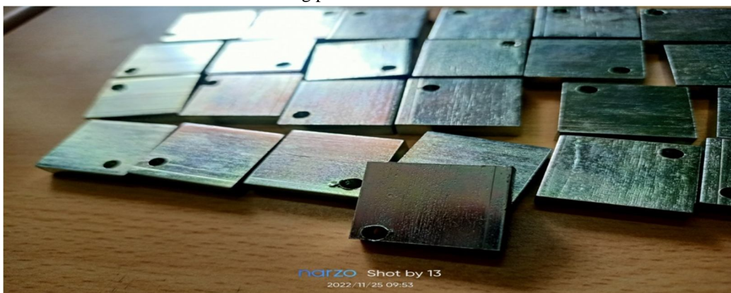
Figure 2. Specimen after zinc plating
