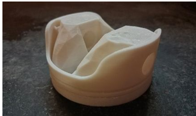
Figure 8 3d printed prototype of the piston
