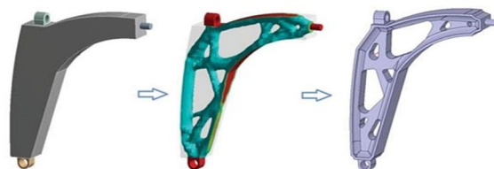
Figure 2: Topology optimization example
