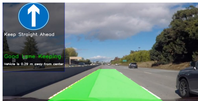
Fig 6: Curved Lane Detection System Showcase
