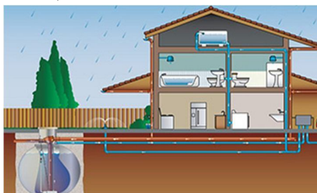
Fig. 1 Rain water harvesting
