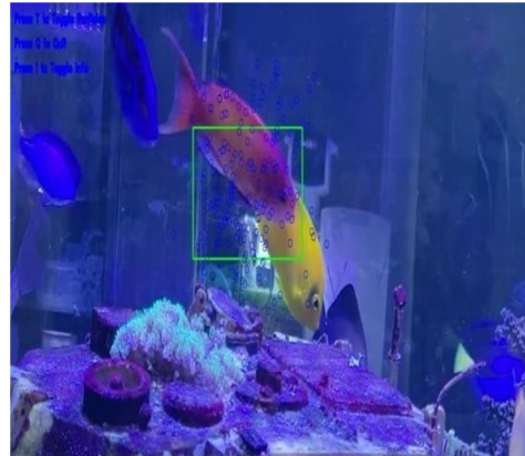
Fig.4. Frame '3': Different coloring methods and histogram comparison involved in tracking of object failed due to multiple objects involvement.
