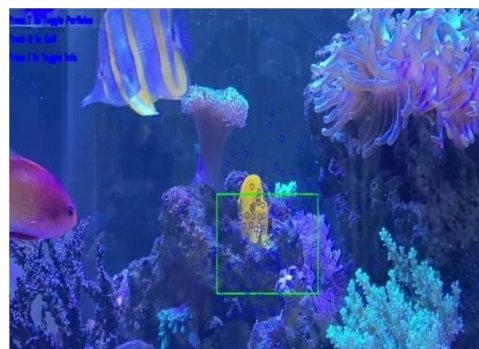
Fig.3. Frame '2': From above two frames object is tracked, But when the object moved from frame '0' to frame '1' the objects motion got distracted due to multiple objects involvement in the video.
