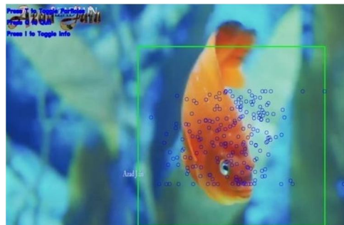
Fig.6. Frame '1': The tracking object is highlighted using color histogram. The rounded bubbles are known as molecules which helps to identify similar colored particles. The similar colored particles are grouped so that tracking of object in under water becomes easier.
