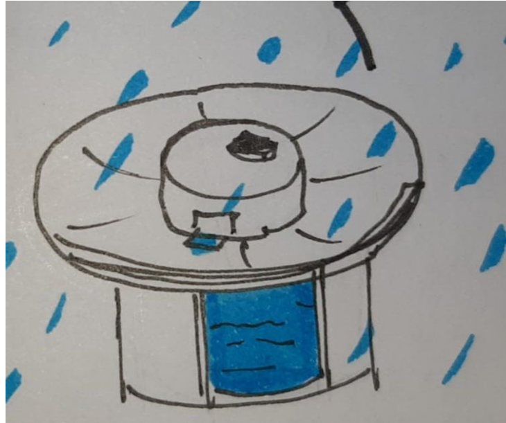
Figure 8: False catchment created for taanka
