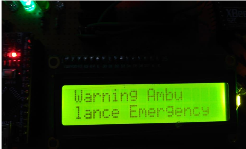
Fig 8: LCD Display when ambulance enters
