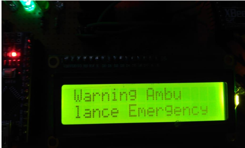
Fig 8: LCD Display when ambulance enters
