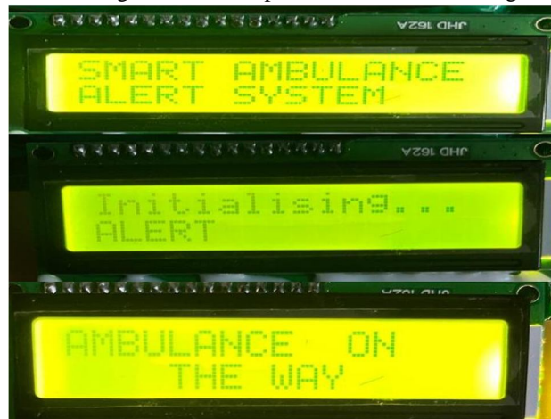
Fig9. Observations on LCD (16*2)Display.
