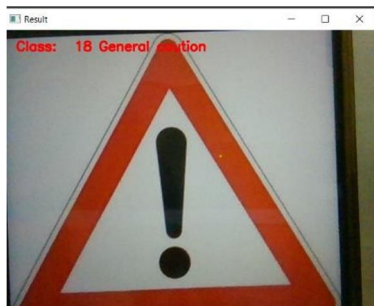
Fig. 11: General Caution sign detected through web cam
