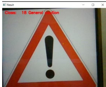
Fig. 11: General Caution sign detected through web cam
