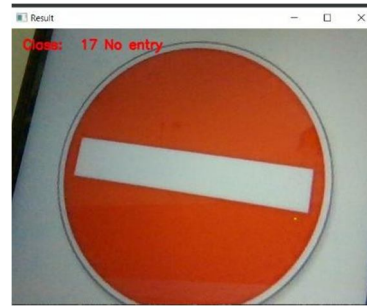
Fig. 12: No Entry sign detected through web cam
