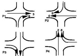
One possible way of providing Four-phase signal
