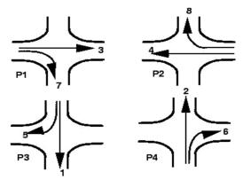
Third possible way of providing Four-phase signal
