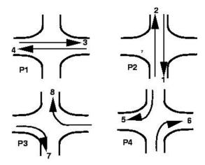
Second possible way of providing Four-phase signal
