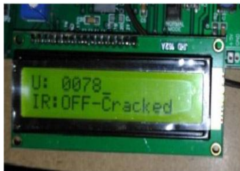
Figure12: Distance from Opposite Vehicle and Crack on Track
