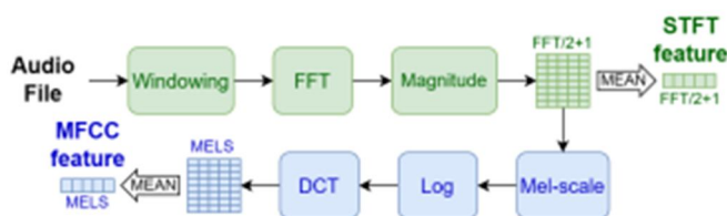
Figure-4: Extraction diagram for STFT and MFCC features.
