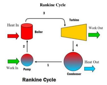
The **Rankine cycle** or **Rankine Vapor Cycle** is the process widely used by <u>power plants</u> such as <u>coal-fired power plants</u> or <u>nuclear</u> reactors. In this mechanism, a <u>fuel</u> is used to produce <u>heat</u> within a <u>boiler</u>, converting <u>water</u> into <u>steam</u> which then expands through a <u>turbine</u> producing useful <u>work</u>. This process was developed in 1859 by Scottish engineer William J.M. Rankine.<sup>[1]</sup>
