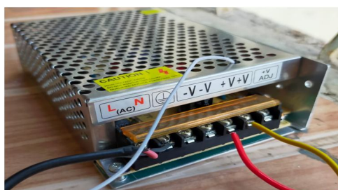
Switched-mode power supply
