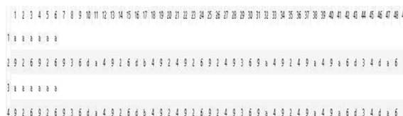
Figure 6 - Demodulated hexadecimal key fob message
