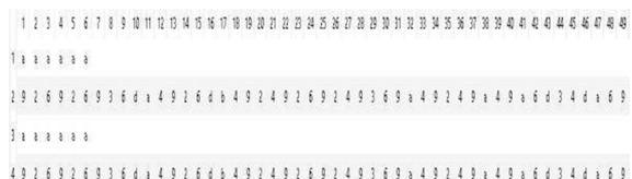
Figure 6 - Demodulated hexadecimal key fob message
