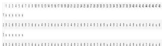
Figure 6 - Demodulated hexadecimal key fob message
