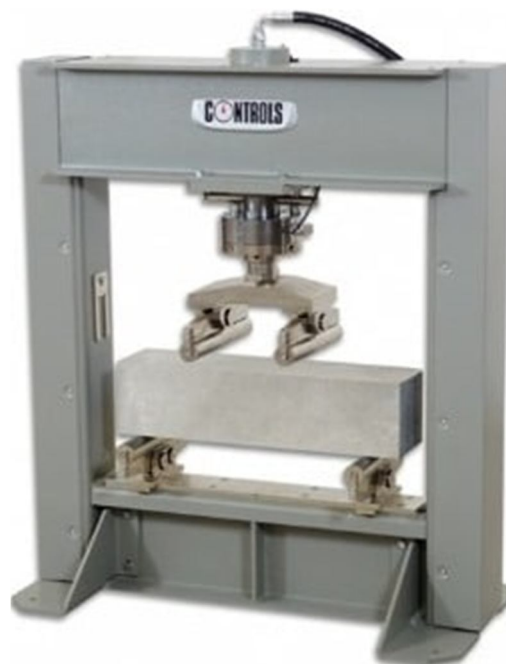
Fig.3.5: Flexural Test Machine and Concrete Specimen (ASTM C78)
