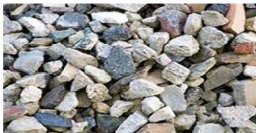
Aggregate from recycled concrete
