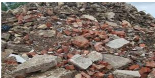
Aggregate from Recycled Demolition Waste
