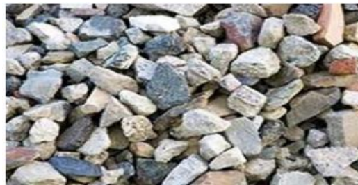
Aggregate from recycled concrete
