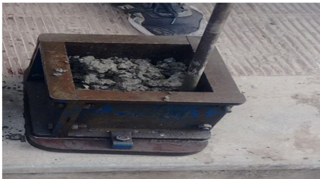
Fig 4.7 Placing of concrete in moulds
