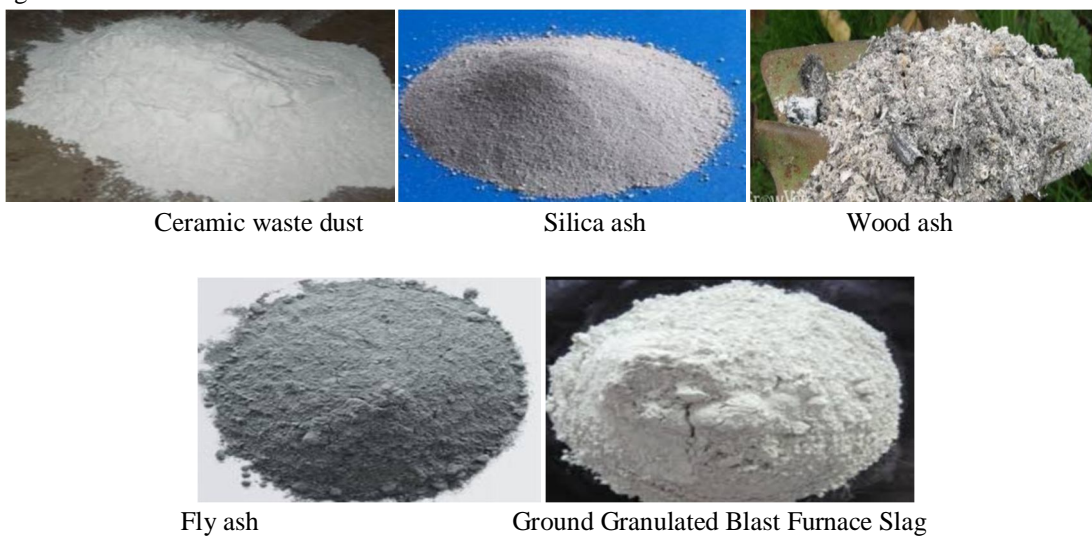
Fig 1.1 Alternatives for partial cement replacement
