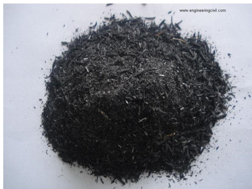
Fig 1.3 Sugarcane Bagasse Ash
