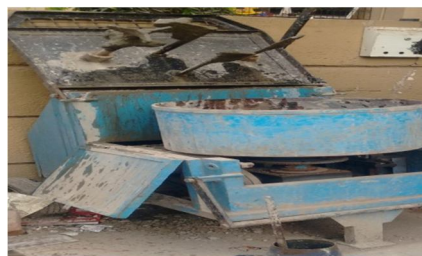
Fig 4.6 Concrete Mixer (Pan type)
