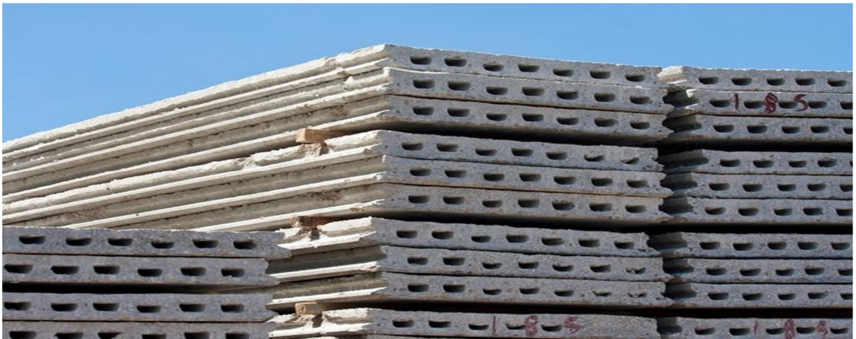
Fig.02 Precast Concrete Slabs
