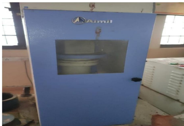
Fig 2.2.3: Compressive strength test of concrete.
