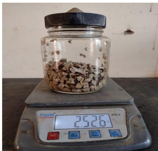
Fig 2.2.2- Specific gravity and water absorption test for tile aggregate.
