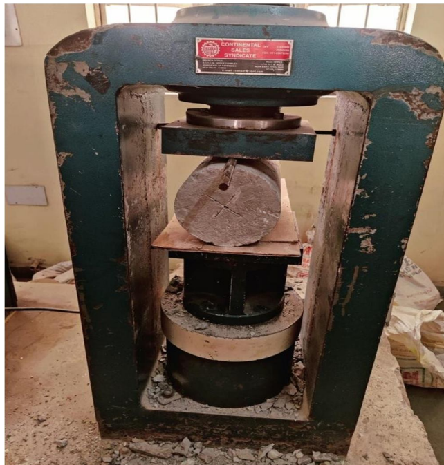
Fig. 2 Compressive Strength of Cylinder
