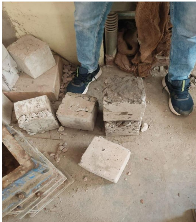
Fig.5 Rubberized Concrete cube cast
