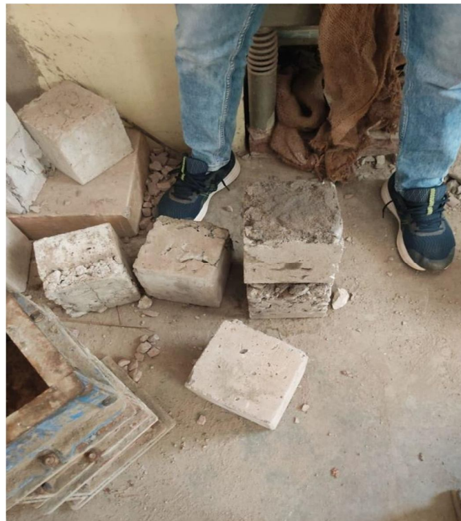
Fig.5 Rubberized Concrete cube cast
