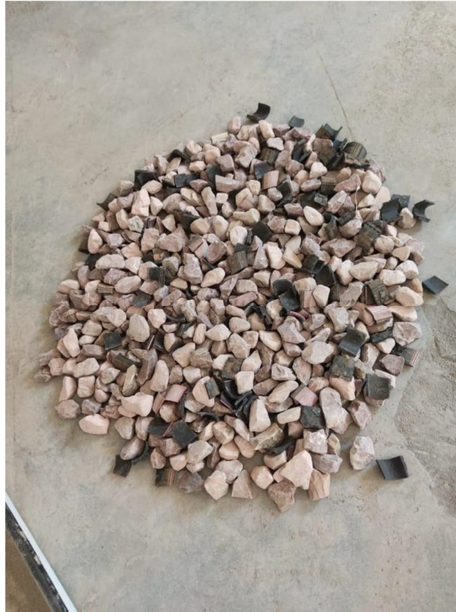
Fig.4 Partial Replacement of aggregates with tyre
