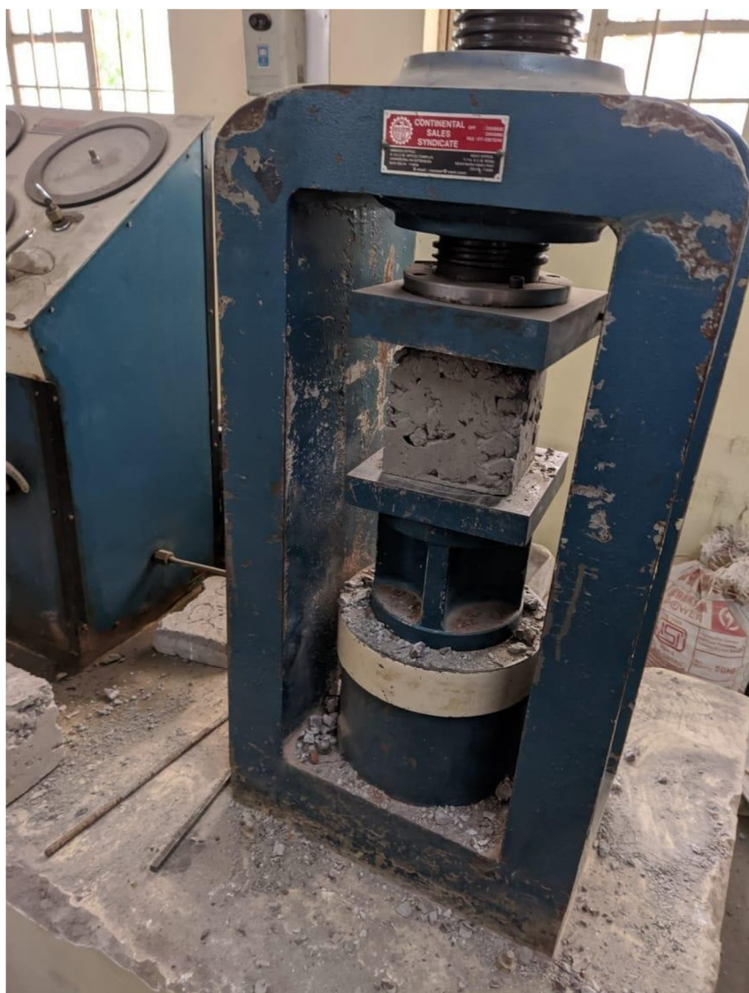
Fig. 1 Compressive Strength Test of Cube
