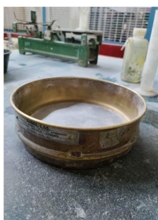
Fig 5.1 90 micron sieve for fineness
