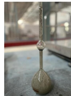
Fig 5.3 Specific Gravity of Cement
