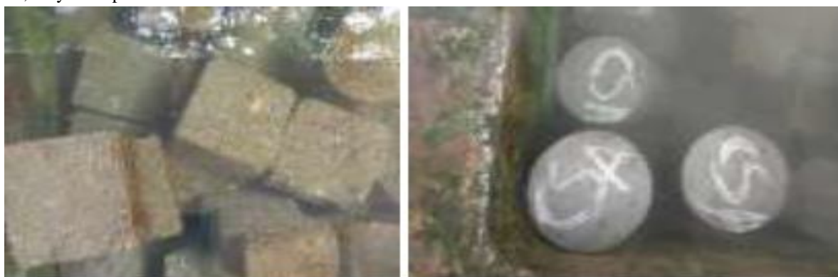
Fig 4.3 :-Curing of cubes and cylinders
