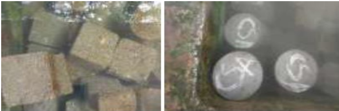
Fig 4.3 :-Curing of cubes and cylinders
