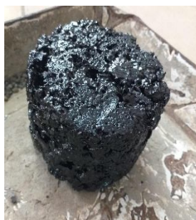
Fig-6: Demoulded Specimens
