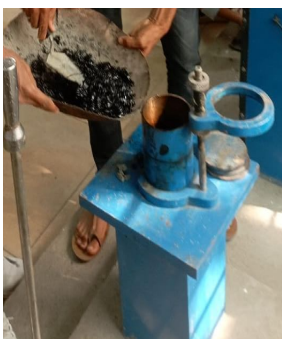
Fig-5: Fill Mix Bitumen in mould
