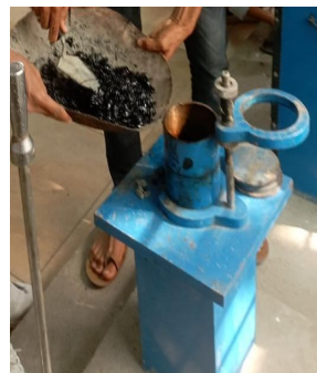
Fig-5: Fill Mix Bitumen in mould
