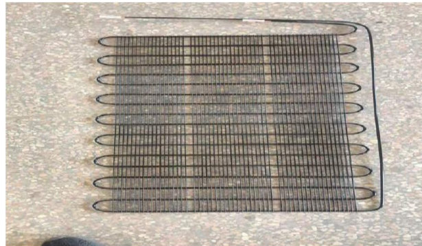
Figure no.3: Condenser
