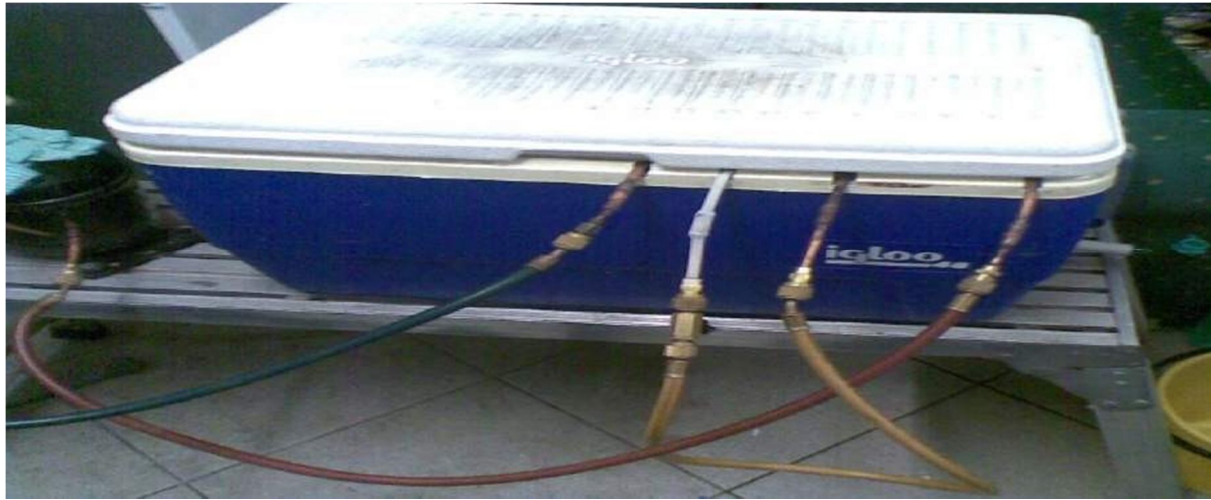
Figure no: 1 Refrigeration Evaporator
