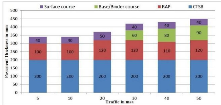
Figure 12.25 Catalogue for pavement with bituminous surface course with CTSB and emulsion/foam bitumen stabilised RAP/virgin aggregate - Effective CBR 5% (Plate-25)
