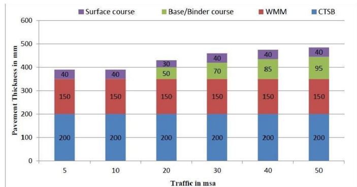
Figure 12.41 Catalogue for pavement with bituminous surface course with CTSB and granular base course - Effective CBR 5% (Plate-41)
