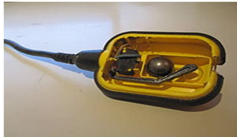
Float switch on
