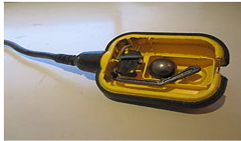
Float switch on
