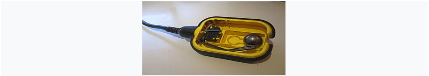
Float switch off
