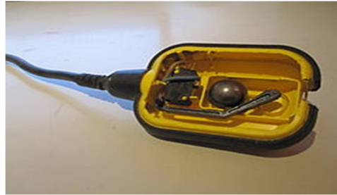
Float switch on
