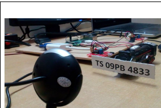
Fig. 7 Image of the number plate being captured by camera
