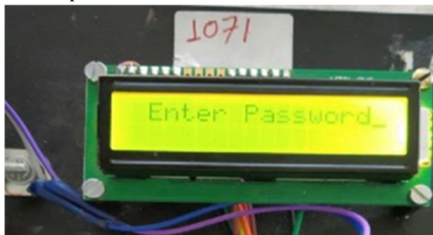
Fig: 3 Display Enter password for unlocking car
