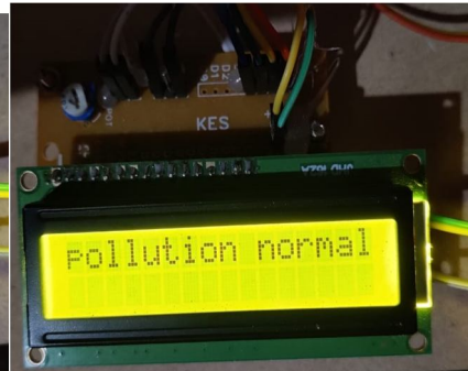
Fig.7: Displaying pollution condition on LCD
