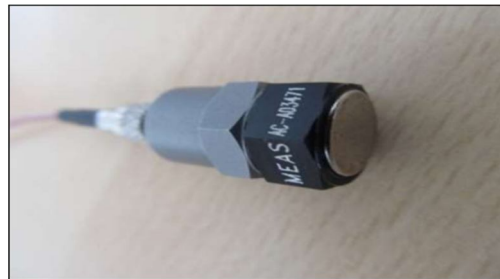
Fig. 9 Accelerometer with Magnetic Base
