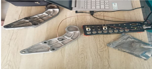
Fig. 7 Aluminium Alloy Engine Mounting Bracket
