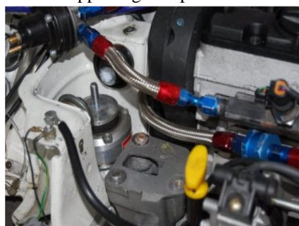
Fig. 2 Position of Engine Bracket
