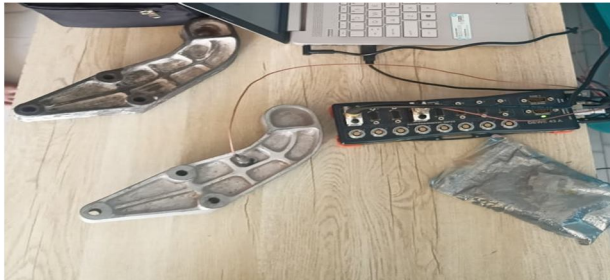
Fig. 7 Aluminium Alloy Engine Mounting Bracket
