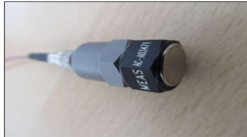
Fig. 9 Accelerometer with Magnetic Base
