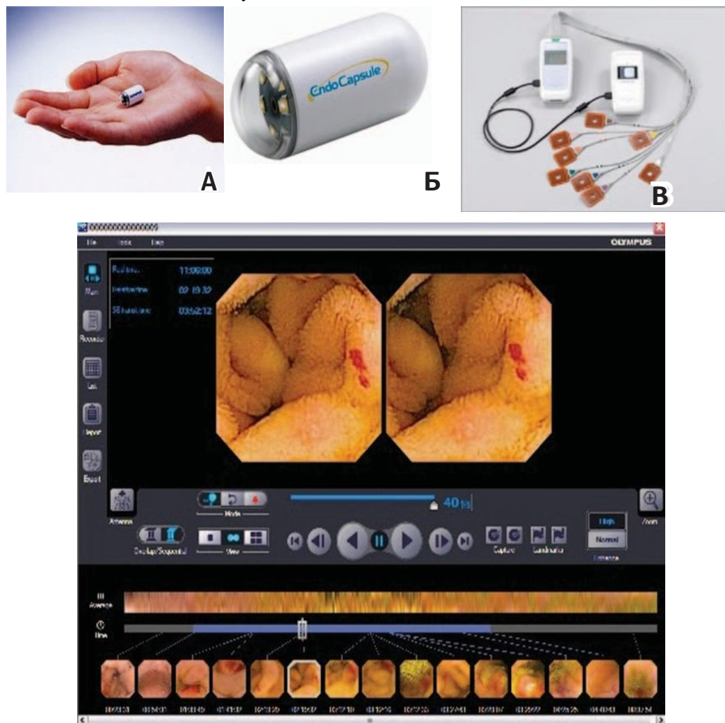
Fig. 1. A – view of the endocapsule, B – endocapsule, C – recording device with attached external antennas and real-time viewer, D – view of the workstation window for viewing and interpreting images
