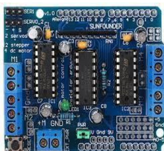
Figure 3: L293D Motor Drive Shield.
