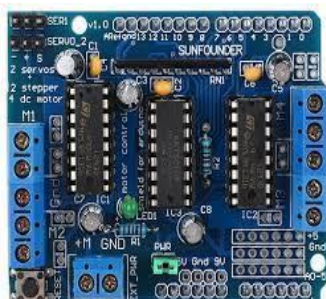
Figure 3: L293D Motor Drive Shield.
