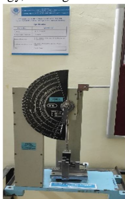
Fig 3. Impact testing machine
