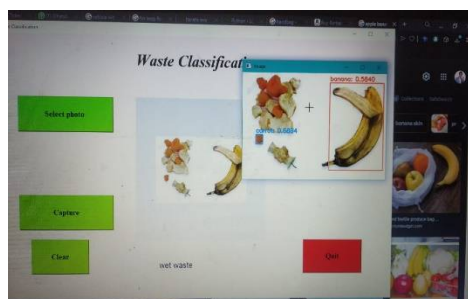
Detection of wet waste using Yolo
