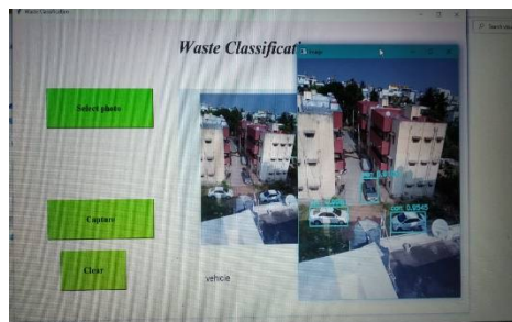
Detection of vehicles using Yolo
