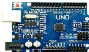
Fig.5 Arduino ATmega 328P Board
