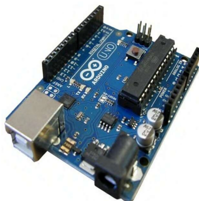
Figure 3: Arduino UNO Board[4]
