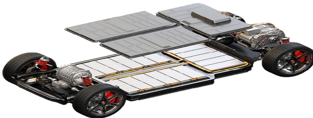
Fig-12: Battery used in an Electric Vehicle
