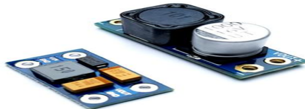
Fig-9: A Standard LC Filter
