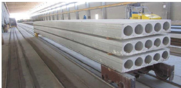
Fig. 1. Hollow core slabs
