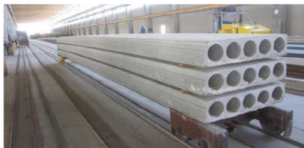
Fig. 1. Hollow core slabs
