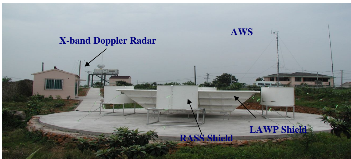
Fig.1 Wind profiler Antenna assembly
